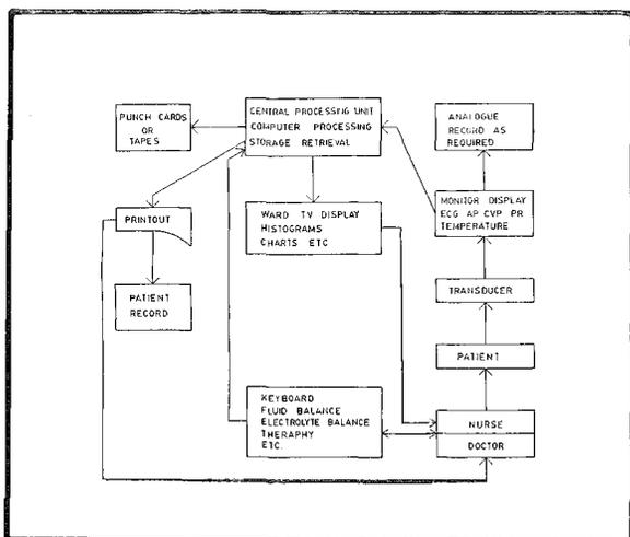
Fig. 2 Block diagram of a computerised patient monitoring system with facilities for automatic and manual data entry. <sup>4</sup>
