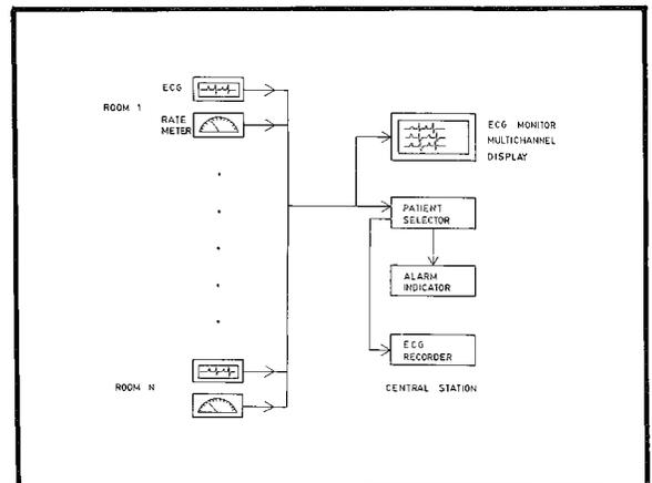
Fig. 1 A typical conventional ECG monitoring system.
