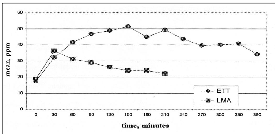
Fig. 1: Graph depicting the changes of nitrous oxide level versus time for both ETT and LMA plotted every 30 minutes.
