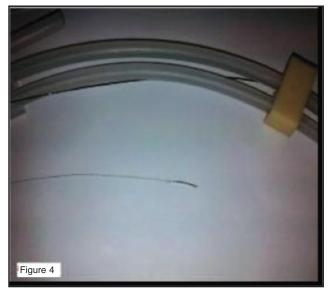
Fig. 4: The stretched out and unraveled distal BMW wire.
