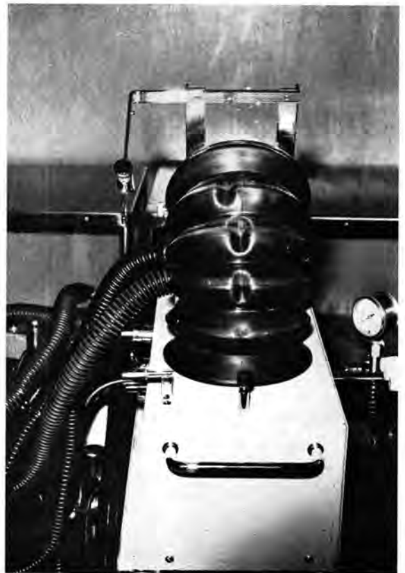
Fig. 1. Manley Ventilator in the failed position, when the arm has slipped from the toggle switch.
